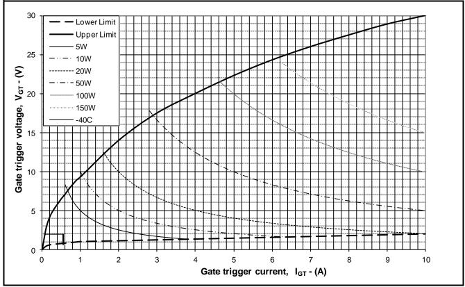
Fig. 15 Gate characteristics
