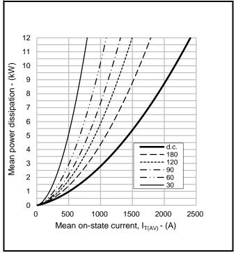
Fig.6 On-state power dissipation - rectangular wave
