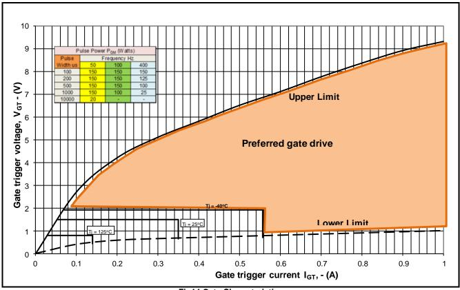
Fig14 Gate Characteristics
