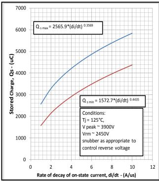
Fig.12 Stored charge vs di/dt
