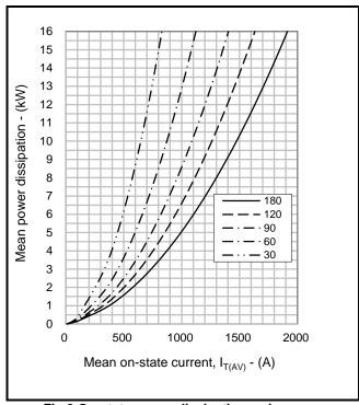
Fig.3 On-state power dissipation - sine wave
