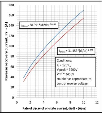
Fig.13 Reverse recovery current vs di/dt
