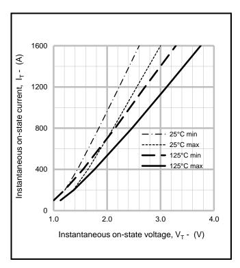
Fig.2 Maximum & minimum on-state characteristics
